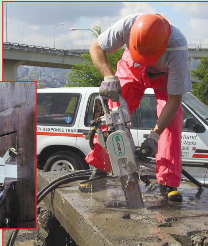
Model CS 71853 11 HP Hydraulic Motor
