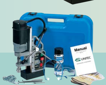
Model ECO-50 with keyless chuck cutter holder
