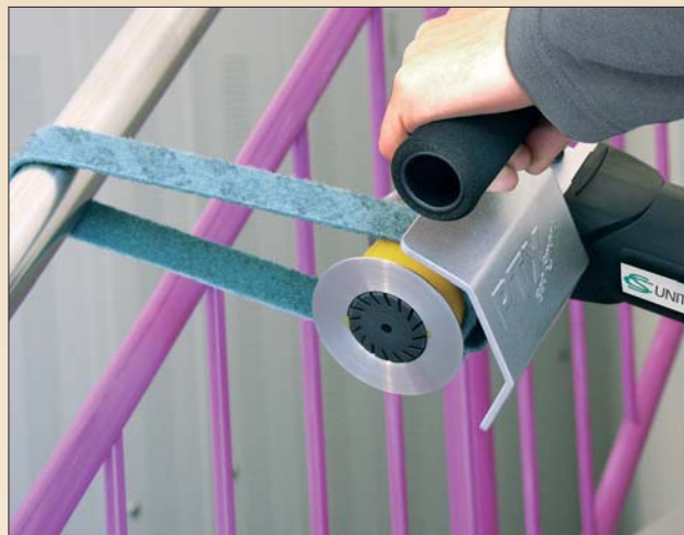
Slide-on grinding belt roller (Part Number 47006) is ideal for open and closed pipe constructions.
